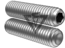
Hexagon socket set screw with cup point DIN916/ISO4029
